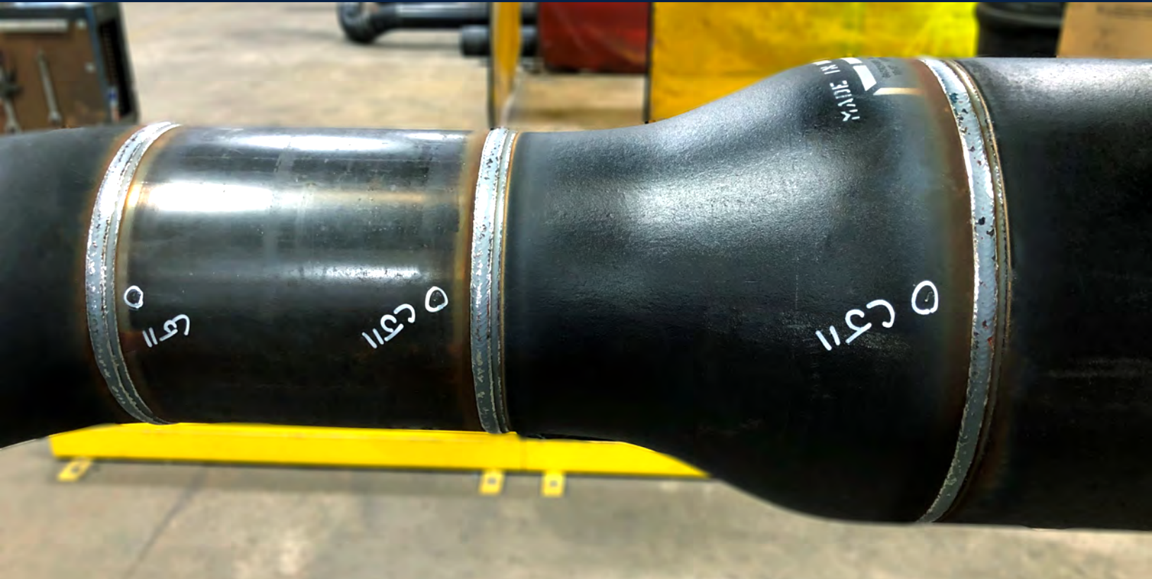
Figure 6: X-ray quality welds performed by the SWR™
